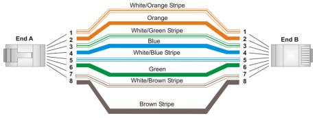
**FIG. 11** RJ-45 wiring diagram
